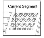
Current Segment column of the matrix. (The incline settings are not shown in the matrix.) The speed settings for the next seven segments are shown in the columns to the right.
